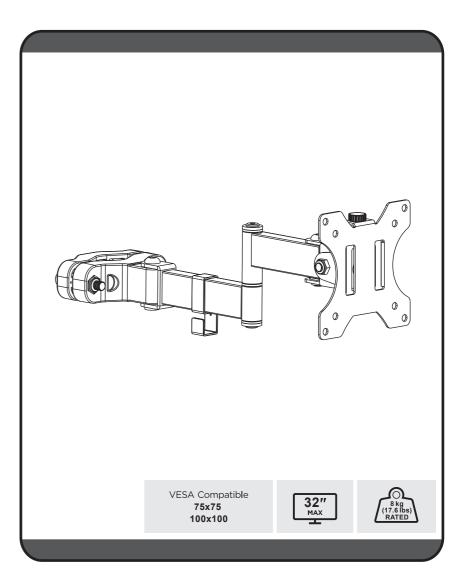
\* The clamp material is made of PC+Glass Fiber, offering high strength and high rigidity. It can withstand strong fastening forces without easily deforming.
