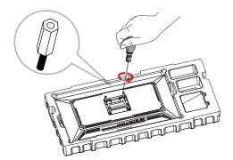
b. Screw the mounting bracket to the VESA holes at the rear of the LCD display.
