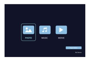
**Note:** The folders in multimedia menu can be opened only if you have connected a USB storage to the LCD display.
