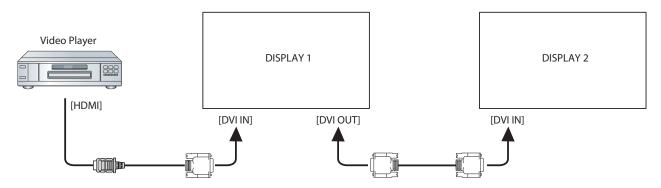
Connect the DVI OUT connector of DISPLAY 1 to the DVI IN connector of DISPLAY 2.
