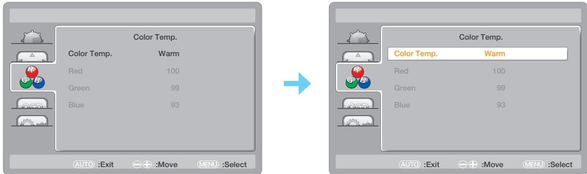
3. Press the  $\wedge$  or  $\vee$  button to select an option and press the
