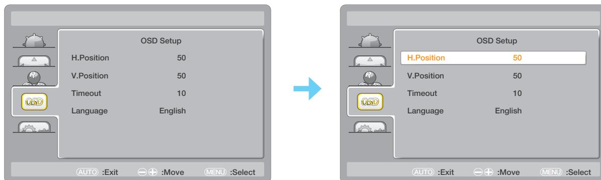
3. Press the  $\wedge$  or  $\vee$  button to select an option and press the
