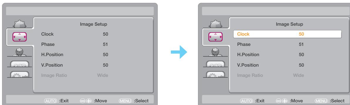
3. Press the  $\wedge$  or  $\vee$  button to select an option and press the
