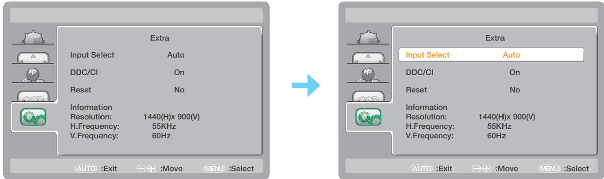
3. Press the  $\wedge$  or  $\vee$  button to select an option and press the
