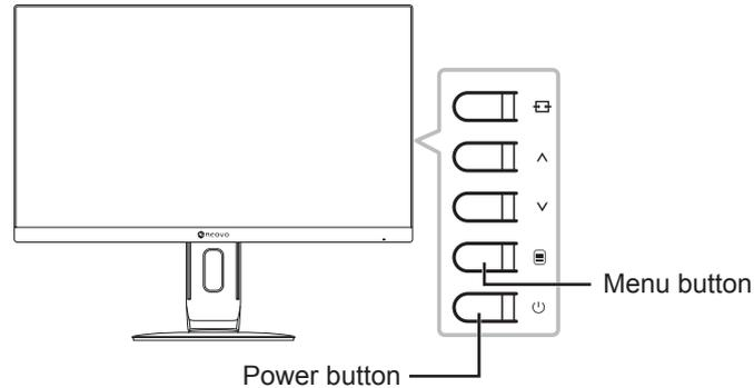
To unlock the OSD menu, press and hold the
