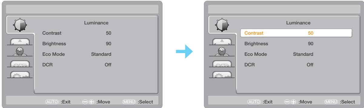
3. Press the  $\wedge$  or  $\vee$  button to select an option and press the
