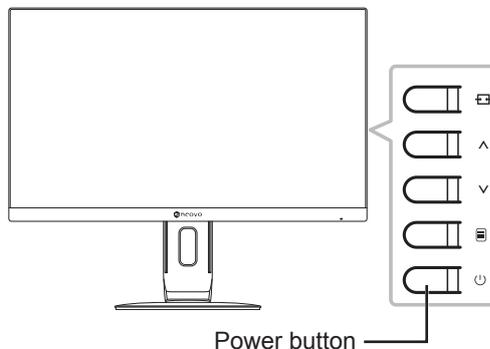
When the LCD display is turned on, press the
