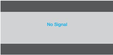
A screenshot of a warning message box with a dark grey header and footer, and a light grey background. The text "No Signal" is displayed in blue.         | The LCD display cannot detect the input source signal.                                   | √ Check if the input source is turned ON.<br>√ Check if the signal cable is properly connected.<br>√ Check if any pin inside the cable connector is twisted or broken. |
