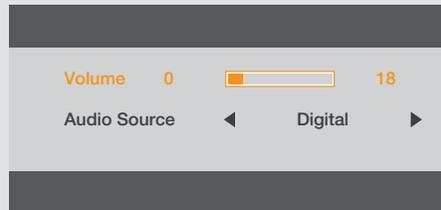
To configure the audio input source, press the
