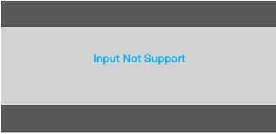
A screenshot of a warning message box with a dark grey header and footer, and a light grey background. The text "Input Not Support" is displayed in blue. | The resolution or the refresh rate of the graphics card of the computer is set too high. | √ Change the resolution or the refresh rate of the graphics card.                                                                                                      |
