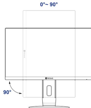
**Note:** Before making the adjustment, make sure to adjust the height to the highest position, and then tilt the screen  $90^{\circ}$ .
