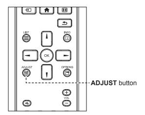
Auto adjustment function automatically tunes the VGA source to its optimal setting, including horizontal position, vertical position, clock, and phase. Press the ††† button. Then press **OK** at the prompt to start the auto adjustment.
