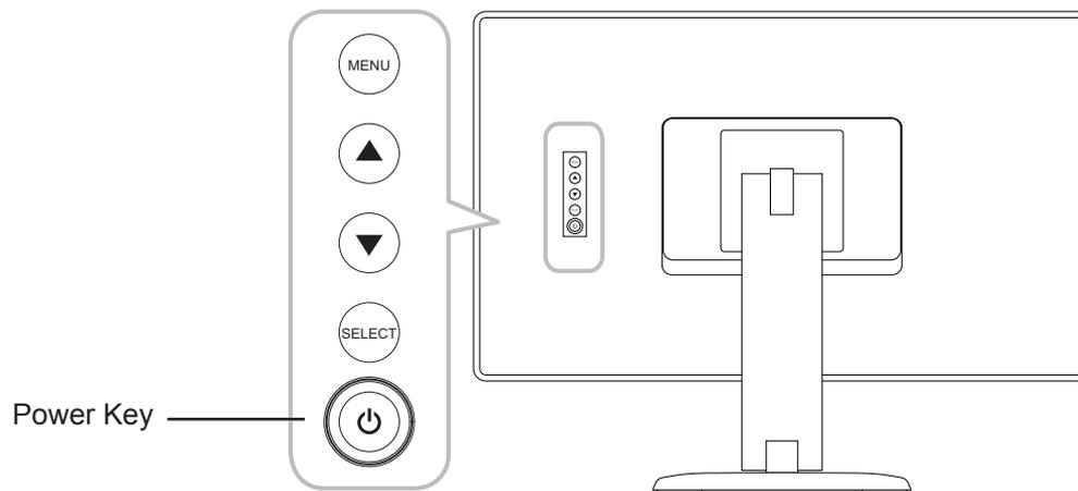
When the LCD monitor is turned on, press the
