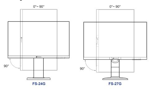
**Note:** Before making the adjustment, make sure to adjust the height to the highest position, and then tilt the screen 90°.
