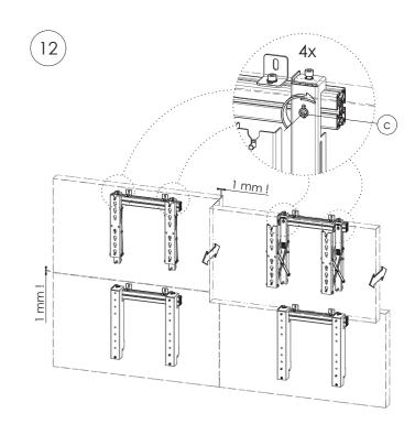
Check virtical position in the push-open and push-closed position and be aware of the 1 mm free space when opening and closing the brackets. Push the screen, mounted on a VWM-02, by pressing against the indicated positions until a slight click is heard. The screen is now locked in the closed position. Turn screws (c) to teight-up the mounts.
