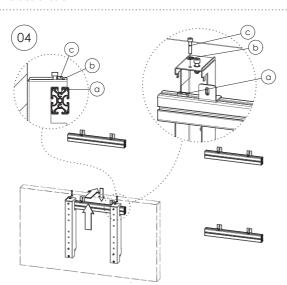
VWM-01: Hook the display with brackets to the aluminium profile and make sure that adjusting screw (c) does not touch the profile.
