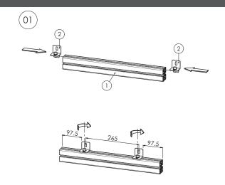
Slide the wallbrackets (2) wit the slot nut in the slot of the aluminium profile (1). Positionate them and sleightly turn on the bolts.
