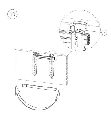
VWM-02: After hanging screen(s) on pushed-out brackets (6) teight-up screws (4) or (5). Keep a distance of 1 mm between 2 screens. Check horizontal positions and fine-tune it by turning screw (e).
