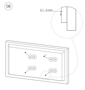
VWM-02: Hook the brackets (6) to the aluminimum profile. Place bolt (a) with associated washer in the sliding nut, fix bracket with bolt (c) into the washer through (b) but do not tighten. Place the two brackets (6) with a horizontal distance according to the width of the VESA and push sleightly on the brackets (6) so they push out. Hang the display in the open bracket (6) by glyding the screws (4) or (5) into the key holes.
